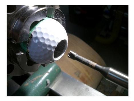
The ball was now hollowed. Just about any type of tool with appropriate reach to under cut inside the ball can be used. Finish is not important here, reducing the weight is. I opted to use a round carbide cutter and removed as much of the interior as I dared. Final weight of the golf ball was less than 30g.
