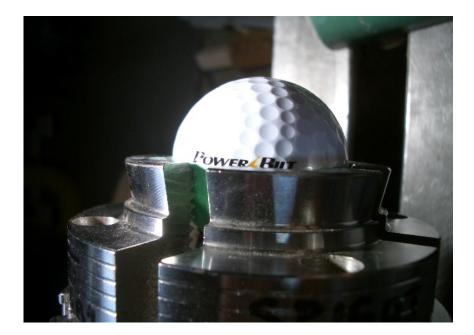
This ball was to be drilled to make the globe part of an ornament. So to keep the top proportionate I opted to drill a 3/4 inch hole in the ball. The hole diameter you drill should match the top you plan on using though. Using a spare ball I gauged the maximum depth of the hole I needed to make to substantially reduce weight and then I put some tape on the Forstner bit to indicate desired depth.
