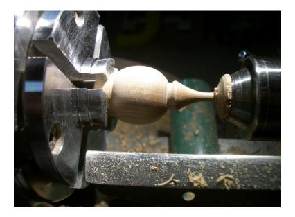
All sanding done under low speed and finish applied (Myland High Friction Polish) at high speed.
