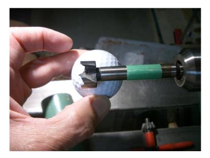
The 3/4 inch hole was then drilled into the ball to the depth required. Remember, this hole was to accept the turned top of the ornament so keep it round when turning. As an aside, apparently the inside of golf balls can be just about any colour...but mine was just an ordinary grey.
