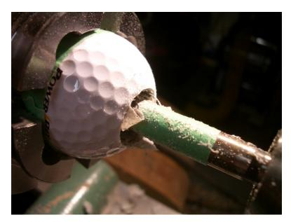
Now, I had to make provision for the 'icicle' part of the ornament to be mounted. Figuring that the Jacob chuck that just drilled the 3/4 inch hole was still concentric to the hole in the ball, I installed a 1/4 inch Forstner bit in the chuck and drilled through the remaining thickness of the golf ball, making a hole to receive the turned icicle. If everything went well this should ensure the top and the icicle are in alignment.
